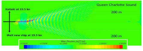
The CFD calculation of wave energy generated by the concept hull shows values between 50% and 70% lower than the maximum allowed wave energy of 9kJ for the range of operating speeds.
