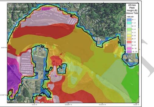
Figure 5 Maximum height above tide map in Newport, Oregon, for a maximum-considered tsunami from Alaska. Note that the Mean Higher High tide is 7.6 feet above geodetic Mean Sea Level (NAVD88). Black lines represents the maximum tsunami inundation. (Figure provided by George Priest, Oregon Department of Geology and Mineral Industries)
