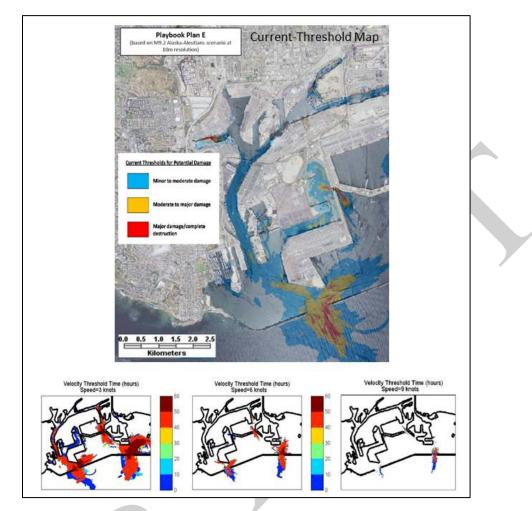
Figure 9 Example of current velocity-damage threshold map (3/6/9 knots), and time-threshold maps for each of the current-damage thresholds in the Port of Los Angeles (modified from the Maritime Tsunami Response and Mitigation Playbook for the Port of Los Angeles, 2015).
