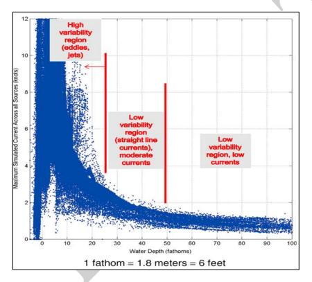
Figure 10 Scatter plot of maximum modeled current velocity versus water depth at Crescent City Harbor (Lynett and others, 2013).
