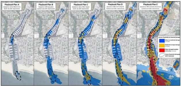
Figure 3 Example maps from Santa Cruz Harbor showing potential damage based on strong currents generated by a tsunamis of different amplitudes (modified from the Maritime Tsunami Response and Mitigation Playbook for Santa Cruz Harbor, 2015). Note the addition of dashed ovals identifying where damaging eddies may form and travel.
