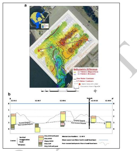
Figure 13 Areas of scour and fill in the Crescent City Harbor Small-Boat Basin determined by differencing multi-beam bathymetric data. The cross section shows the post-tsunami sediment composition and correlation between tsunami and non-tsunami deposits (from Wilson and others, 2013b).
