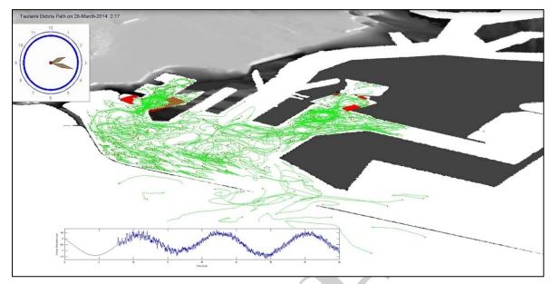
Figure 14 Modeled debris/particle movement from small-boat basins within the Port of Los Angeles (Lynett, unpublished).
