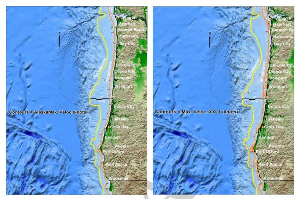
Figure 11 Maximum tsunami current maps for a modeled large Alaska scenario and a large Cascadia scenario (Oregon MAC, 2013).
