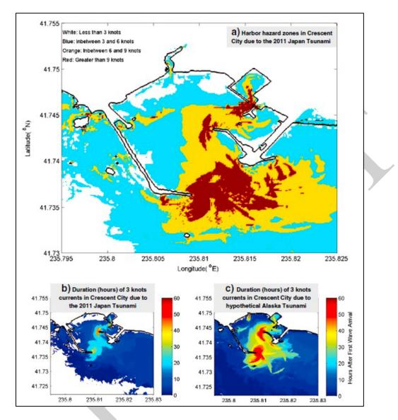
Figure 8 Example uses of the current speed hazard zones for 3/6/9 knot zonation, and time-threshold maps for two different sources in Crescent City Harbor (from Lynett and others, 2013).
