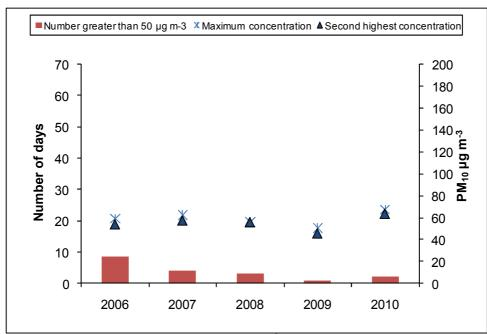
Figure 3.8: Number of days when 50  $\mu$ g m<sup>-3</sup> was exceeded, the maximum concentration and the second highest concentration from 2006 to 2010.
