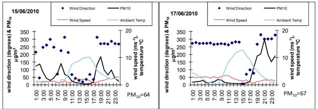
Figure 3.9: Hourly average wind speed, wind direction and temperature on days when  $PM_{10}$  concentrations exceeded 50 µg m<sup>-3</sup> (24 hour average) at Blenheim.
