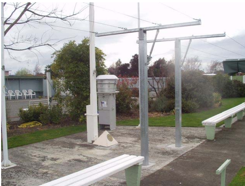
Figure 2.5: PM 10 monitor at the Redwoodtown - Bowling Club air quality monitoring site (note picture depicts high volume sampler but indicates current location of the BAM).
