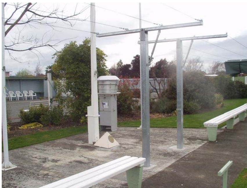
Figure 2.5: PM 10 monitor at the Redwoodtown air quality monitoring site
