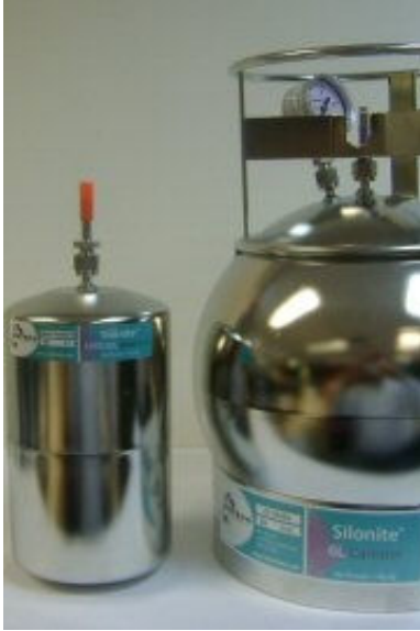
Photo 1: Gas canisters (1.4L and 6L)
