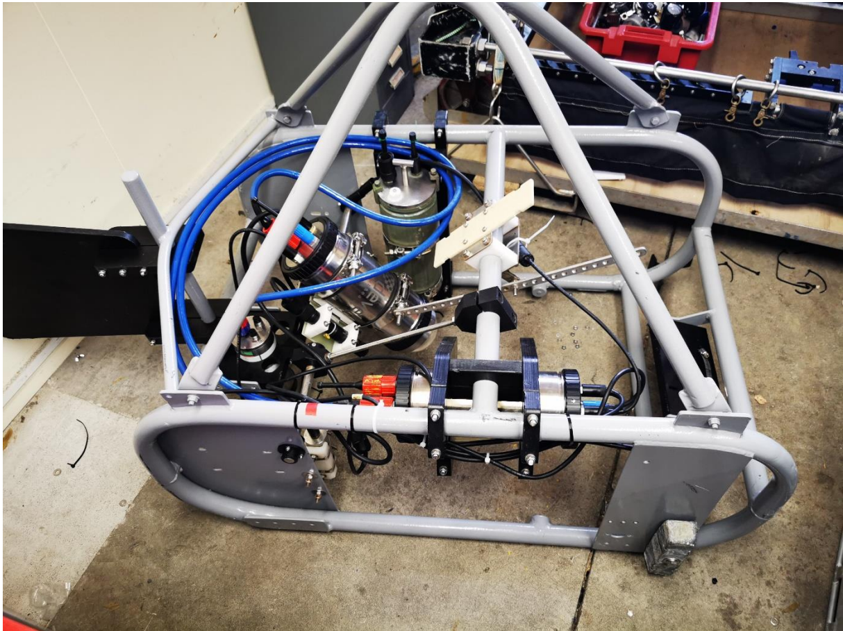
Figure 4-3: NIWA's CoastCam benthic imaging system. The system uses high-resolution 4K and 1080p video and a fibreoptic umbilical cable to relay imagery as a live feed directly to the vessel.
