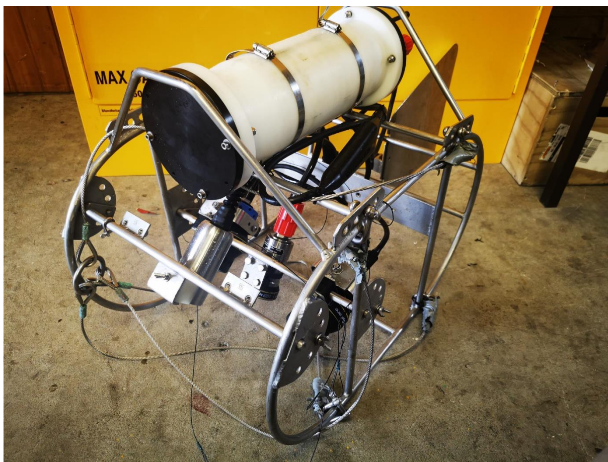
Figure 4-4: NIWA's high-definition CBed camera system. This unit is smaller and lighter than CoastCam and was ideal for towed mid-water surveys along marine farm lines.
