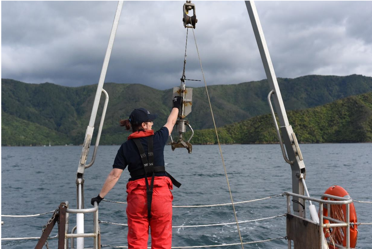
Figure 4-2: Dietz-Lafond (clam-shell) grab being deployed through the aft A-frame of RV Ikateri . Note the spring-loaded jaws in the open position, which will shut rapidly on contact with the seafloor.
