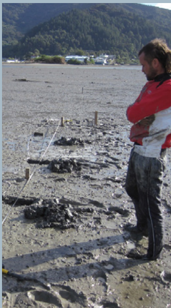
Installing sediment plates at Site D in 2015.
