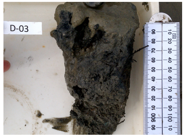
Photo 4-7: Representative samples indicative of relatively shallow (0.5-1 cm) apparent Redox Potential Discontinuity (aRPD) depths at each fine scale site in 2019.
