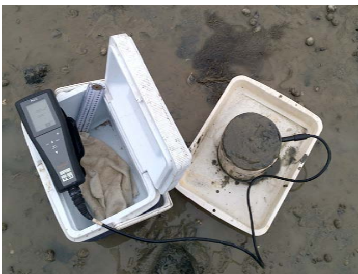
Photo 8-9: Sampling equipment used to measure down-core (0-10 cm) redox potential (mV), a proxy for sediment oxygenation, at each fine scale site, Havelock Estuary, 2019.
