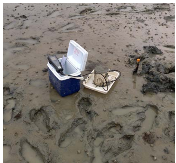
Photo 8-9: Sampling equipment used to measure down-core (0-10 cm) redox potential (mV), a proxy for sediment oxygenation, at each fine scale site, Havelock Estuary, 2019.
