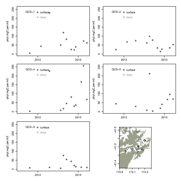
Figure 4-38: Time-series of phytoplankton carbon (mg C m<sup>-3</sup>) measured at five sites in Queen Charlotte Sound. Carbon concentration was derived from cell counts and cell dimensions.
