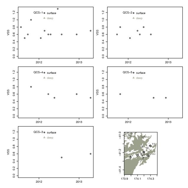
Figure 4-37: Time-series of volatile suspended solids (g AFDW m<sup>-3</sup>) measured at five sites in Queen Charlotte Sound.
