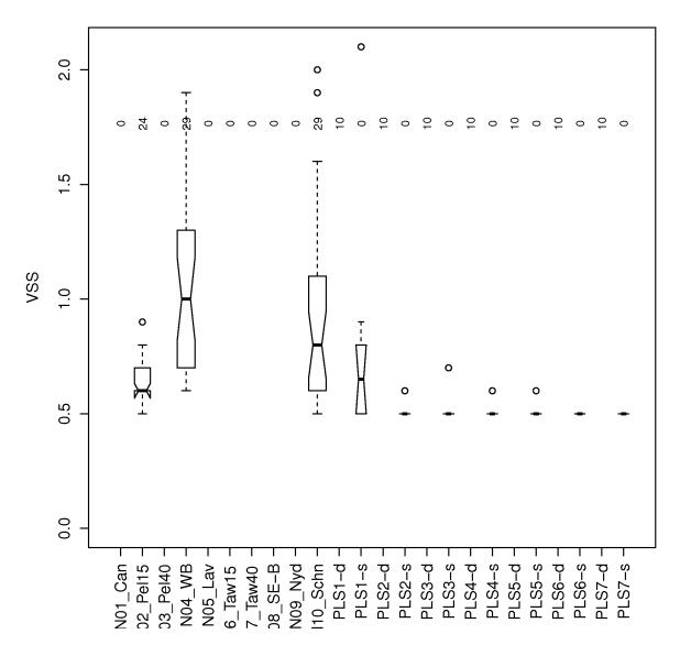
Figure 4-25: Boxplots illustrating the distributions of all volatile suspended solids concentrations (g AFDW m<sup>-3</sup>; over the entire length of each time-series) in NIWA's (N01-N10) and MDC's (PLS-1-PLS-7) Pelorus Sounds data. VSS concentrations recorded as <0.5 g m<sup>-3</sup> by the laboratory were scored as 0.5 g m<sup>-3</sup> in this analysis.
