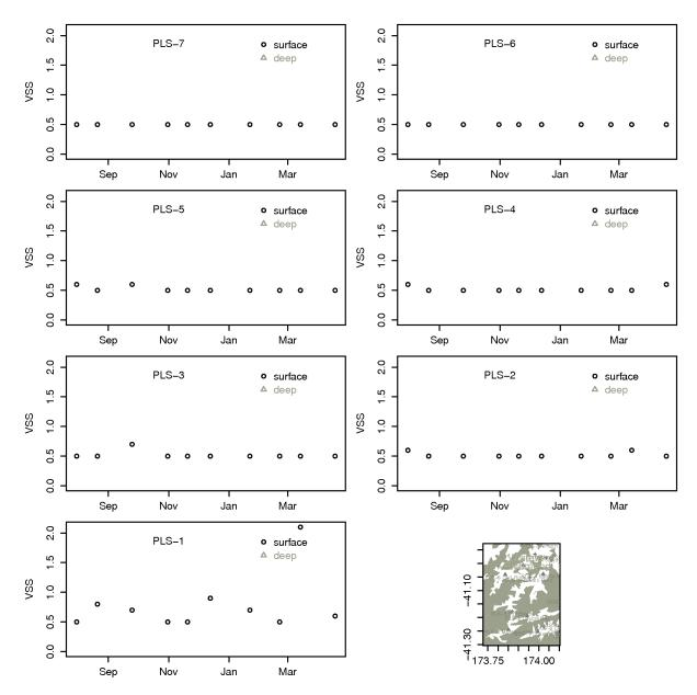
**Figure 4-13:** Time-series of volatile suspended solids (mg AFDW m<sup>-3</sup>) measured at seven sites in Pelorus Sound in the Marlborough District Council sampling program (2012-2013). Values showing as 0.5 on the graphs are recorded as <0.5 in the laboratory reports. Thus, the points on the graphs are over-estimates of the true concentrations.
