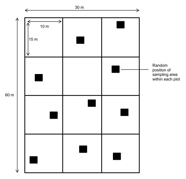
Figure 2 Grid sampling design for the fine-scaling monitoring
