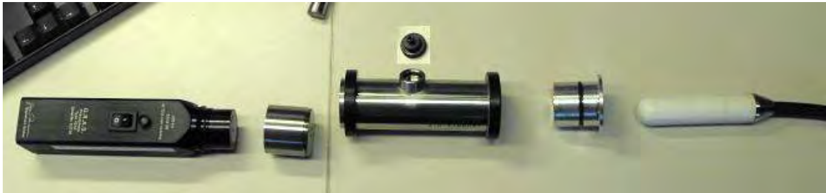
Figure B-1. Split view of (left) a GRAS pistonphone calibrator, (middle) adapters, and (right) a hydrophone.
