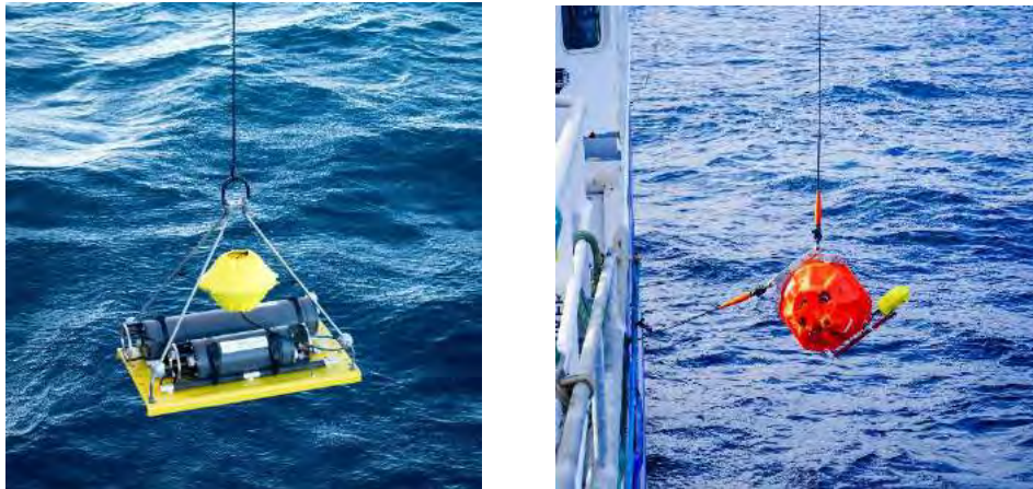
Figure 3-1: JASCO Acoustic Multichannel Acoustic Receivers (AMAR). On a bottom base plate for shallow water deployments at stations 1-3 (left) and housed in a glass sphere for deep water deployments at stations 4-7 (right).
