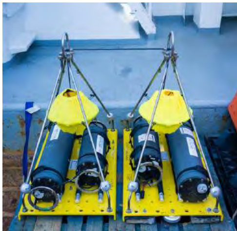
Figure 2. JASCO AMARs on baseplates prior to deployment at Station 2 and 3 by NIWA, June 2016 (Image Credit: NIWA).
