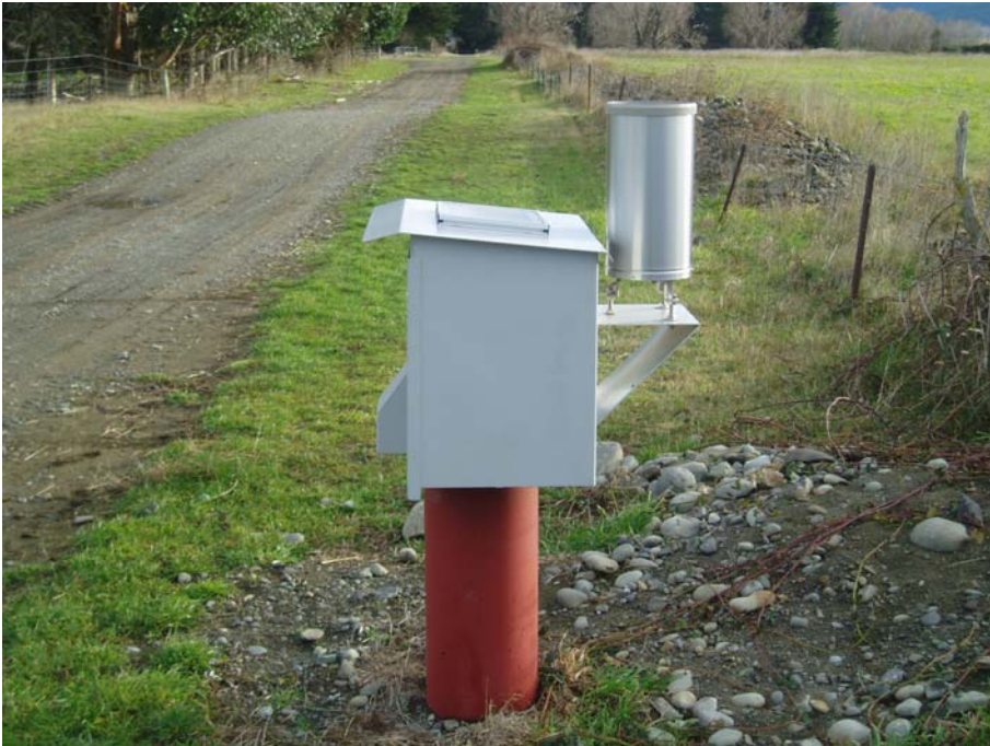
Figure 10: MDC Wairau Valley Aquifer Level Recorder at Mill Road
