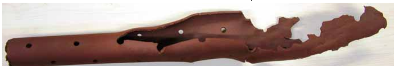
Figure 3.6: Blown-off well pipe. Note the round drilled holes in the pipe which allow water into the well.
