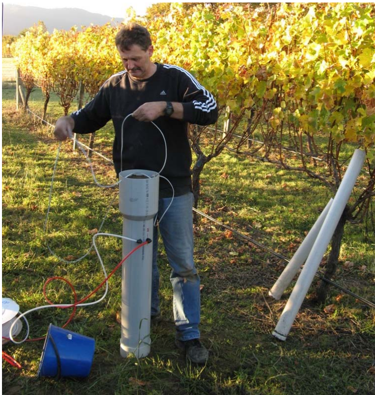
Figure 6: Steve Green from Plant & Food Research is preparing a drainage flux meter (DFM) for installation into the soil at Motukawa vineyard near Raupara, Blenheim. The top 20 cm of this DFM has been filled with soil from a depth of 1.0–1.2m.
