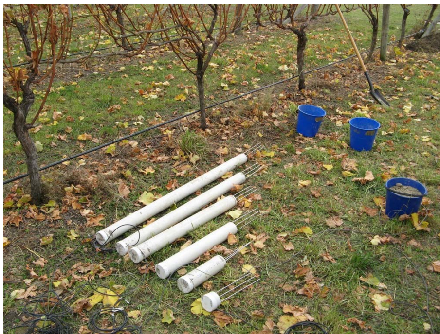
Figure 10: An array of 30cm long TDR (time domain reflectometer) waveguides that are being used to measure changes in the soil water content to a depth of 1.8 m beneath the vineyard. A 10 cm diameter hole was augured to the correct depth, then the TDR probe was inserted into the hole, with the 3-wire waveguides being placed into undisturbed soil.
