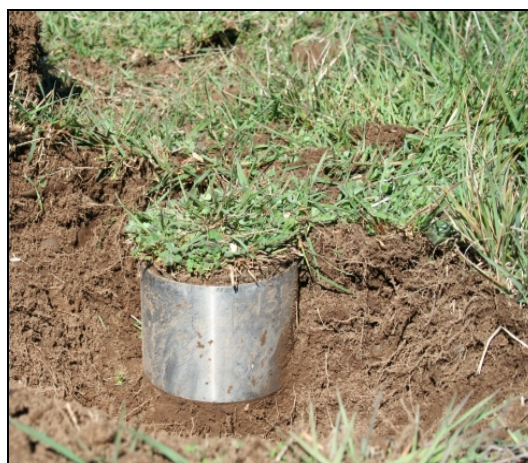
Figure 1(a). Collecting a composite of core samples along a transect using a soil corer (b) One of three intact core samples taken at each site to establish the physical properties of the soil.
