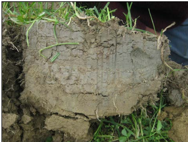
Figure 2. An undisturbed vertical block of soil collected for aggregate stability analysis.
