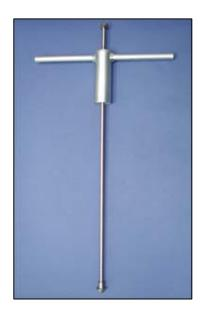
Figure 10 AgResearch penetrometer used to test soil strength before cows enter a paddock
