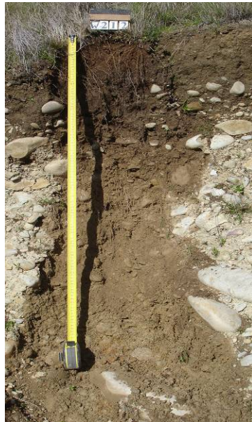
Figure 8. Waihopai hill soil with a thin (25 cm) loess cover and a yellowish brown B Horizon passing into olive brown in situ gravel at 100 cm.
