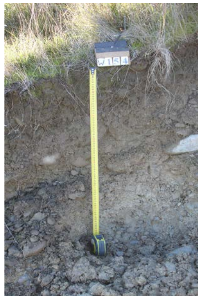
Figure 14. Waihopai hill soil on a lower slope with subsoil grey colours indicating drainage impedance. Reworked material lies over in situ firm saturated gravel on which a slip has occurred.
