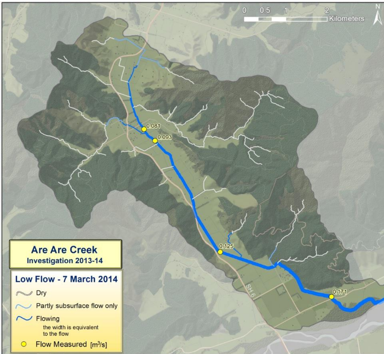
Figure 4: Summer low flow gaugings on 7 March 2014.
