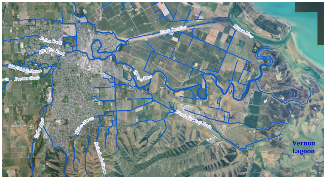
Figure 25: The main network of drains in Blenheim which ultimately discharge to the Vernon Lagoon.
