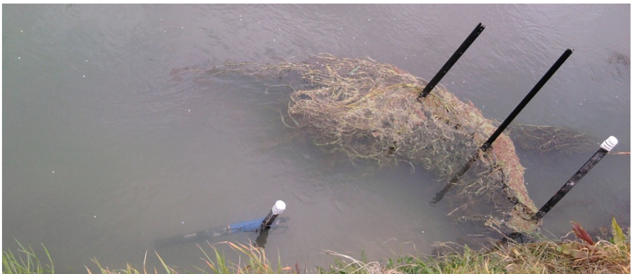
Figure 46: The 'Sonde' used for the continuous monitoring deployed in Fairhall Coop Drain. The screen to the right prevents floating aquatic weed to accumulate on the instrument.
