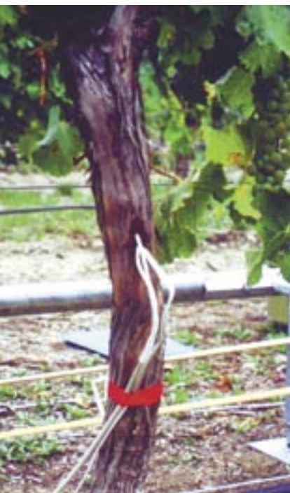
Heat pulses measure water movement in a grape plant
