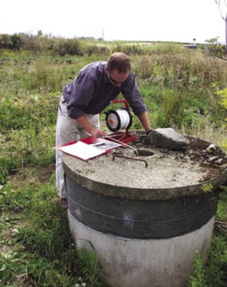
Monitoring ground water levels
