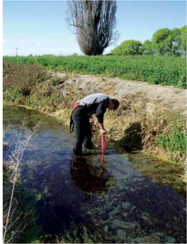
Piezometer being used in Dowlings Creek to measure aquifer level relative to spring level
