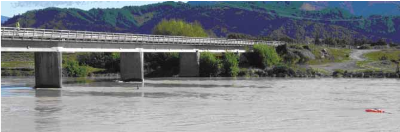
The Rio Grande Acoustic Doppler Current Profiler deployed for flood gauging, using a tagline from the Wairau Diversion bridge
