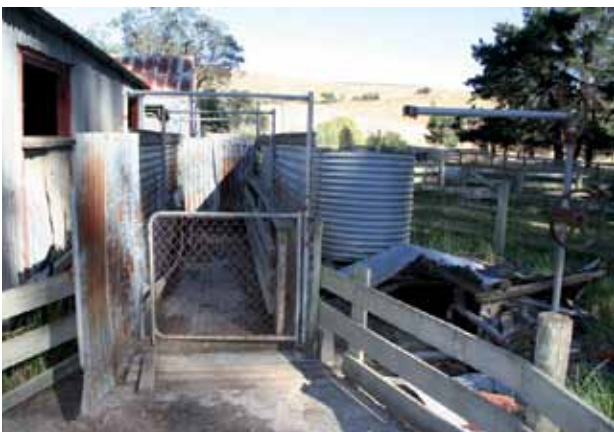
Disused power-spray machine used to treat sheep for parasites with chemicals such as arsenic dieldrin and DDT
