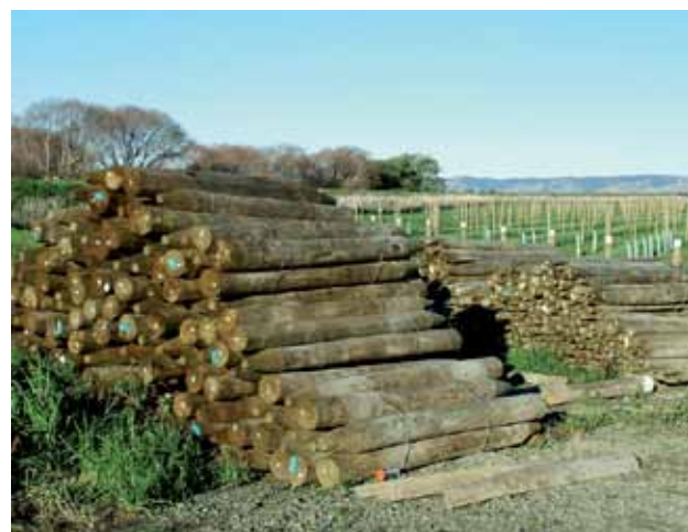
Copper, chromium, arsenic treated vineyard posts stacked and ready to be used in the field
