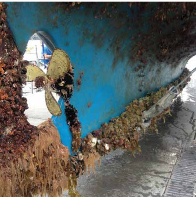
Heavily fouled yacht with Mediterranean fanworm found in Waikawa Bay, 2014. Vessel hulls should be inspected and cleaned regularly to prevent infestations and spread
