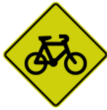
Figure 4-1: PW-35 Cyclists sign
