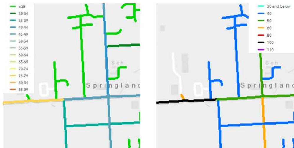
Figure 2-7: Mean Operating Speed and Safe & Appropriate Speed (source: MegaMap)
