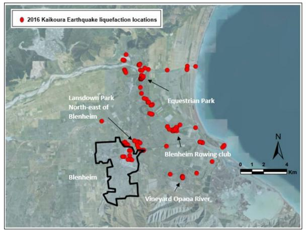
*Figure 2 Locations of liquefaction manifestation from the 2016 Kaikōura Earthquake*<sup>1</sup>.
