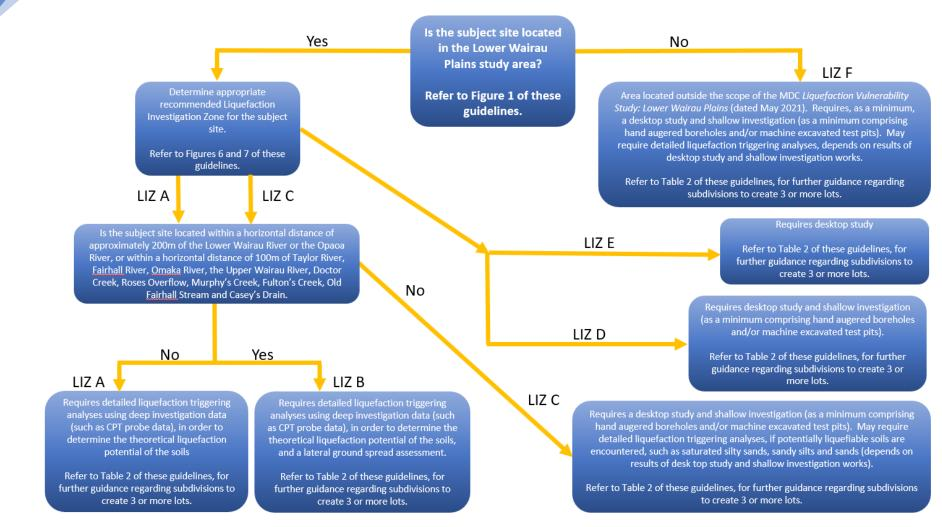
Figure 8 Flowchart: Determination of suitable geotechnical investigations for liquefaction potential assessment purposes (general).
