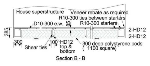
The ground immediately beneath the polystyrene and ribs must have a minimum geotechnical ultimate bearing strength of 200 kPa, or the system should be subject to specific engineering design (refer to section 3.4.1). Shear ties in accordance with NZS 3101 are required in the ribs.
