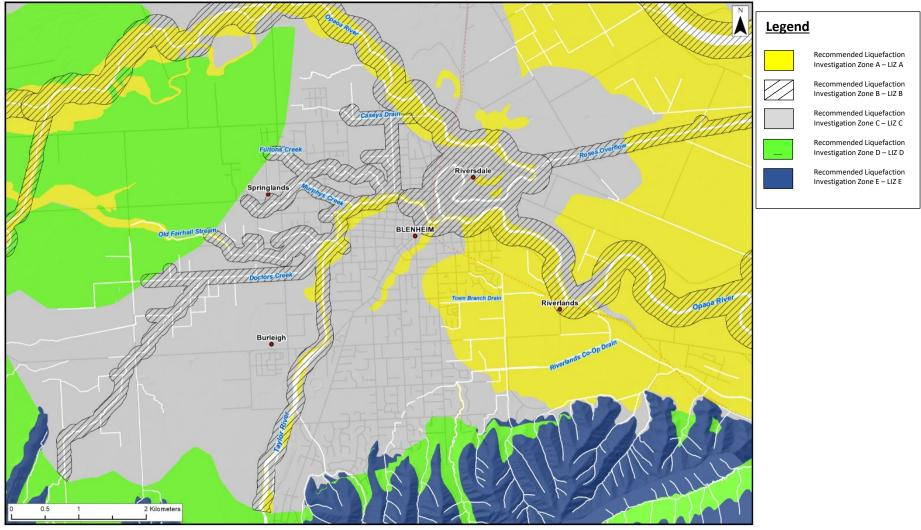
*Figure 7 Liquefaction Investigation Zones (LIZ) for the Lower Wairau Plains – Blenheim Area.*
