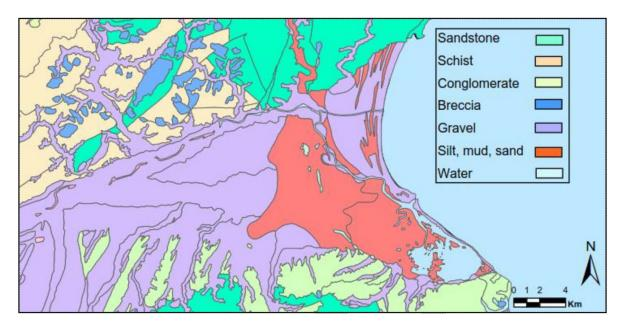
Figure 3 Surface geologic map of the Lower Wairau Plains<sup>2</sup>.
