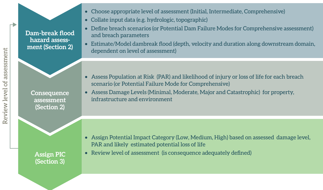
Figure 1.1: Overview of the Dam Classification Process
