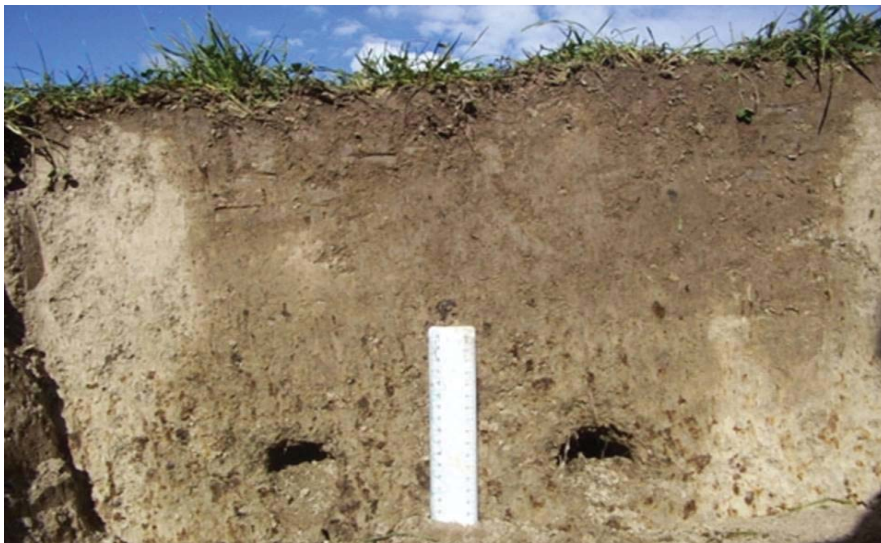
Figure 5. Field example of preferential flow through a Pallic soil containing remnants of old mole drains.
