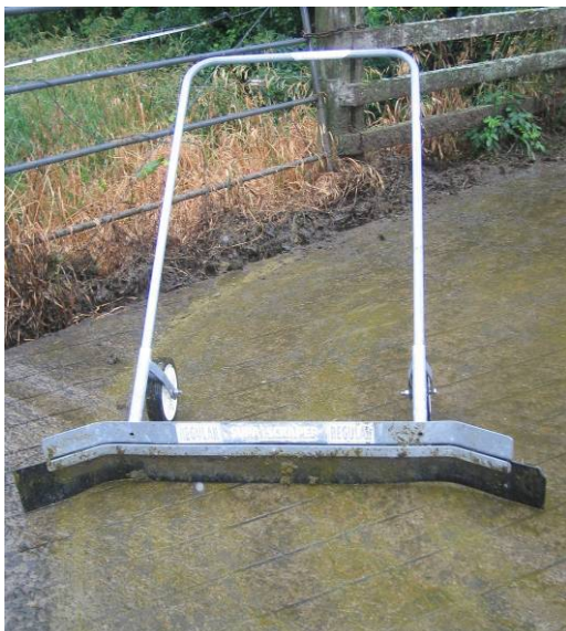
Effluent scrapers minimise water use, which minimises the volume of effluent to be disposed of.
