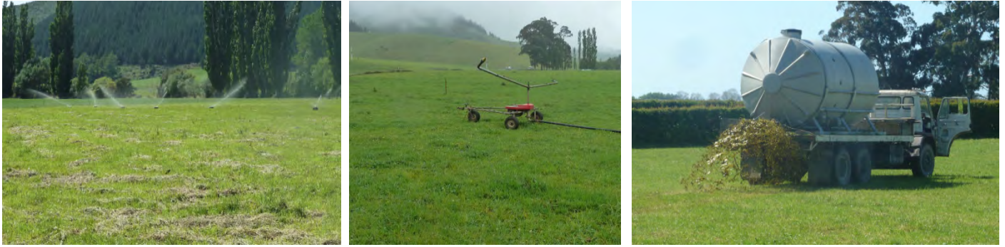
The most common types of effluent disposal in Marlborough from left to right; k-line pods, travelling irrigator and spreader truck
