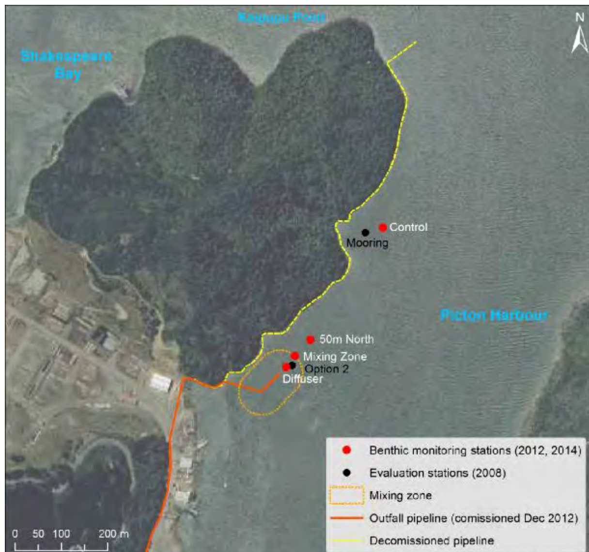
Figure 1. Map of Picton Harbour indicating locations of current and previous benthic sampling stations and the current and decommissioned outfalls from the Picton wastewater treatment plant.
