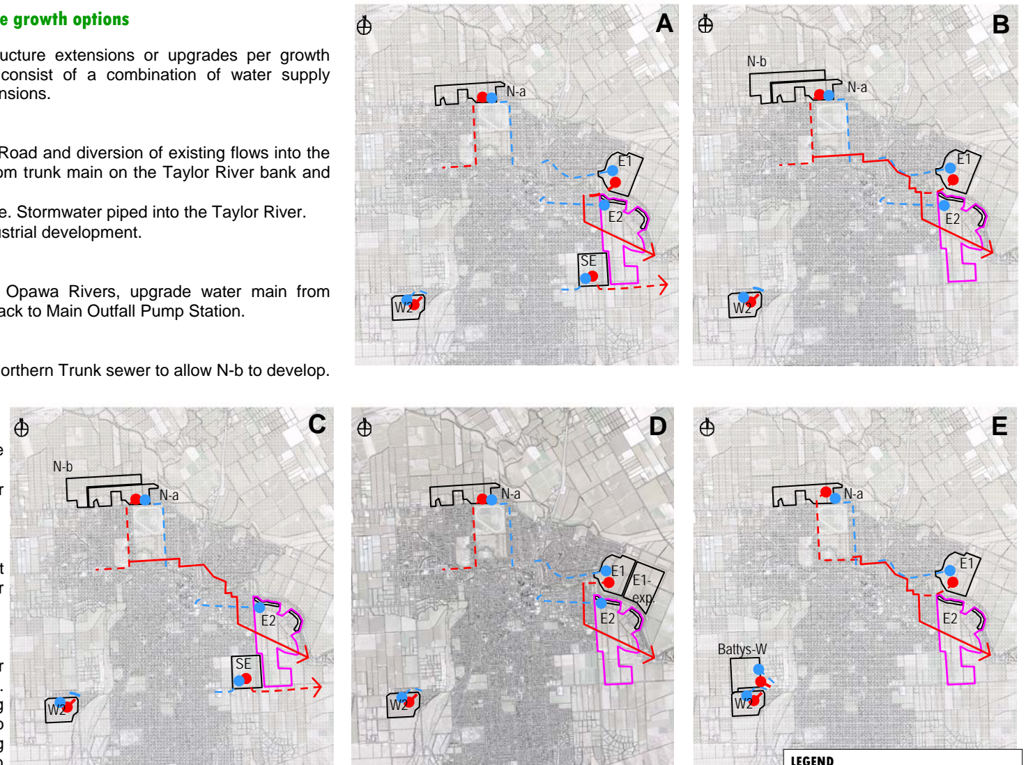
ABOVE FIG. 6-30: Growth options A, B, C, D and E, with their respective implications for water supply and sewerage infrastructure.
