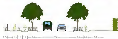
ABOVE FIG. 5A-9: Option 2 Proposed kerb build-out High and Havelock Streets. Off-street cyclists outside the build-outs
