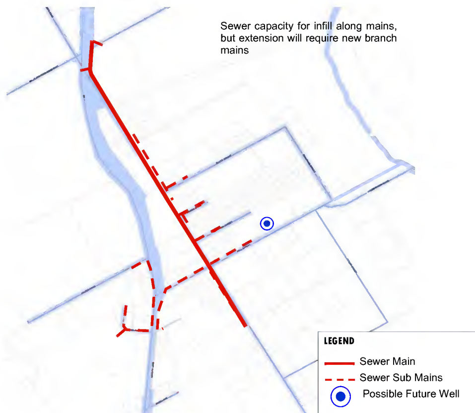
LEFT FIG. 5C-6: Sewer & Proposed Well.
