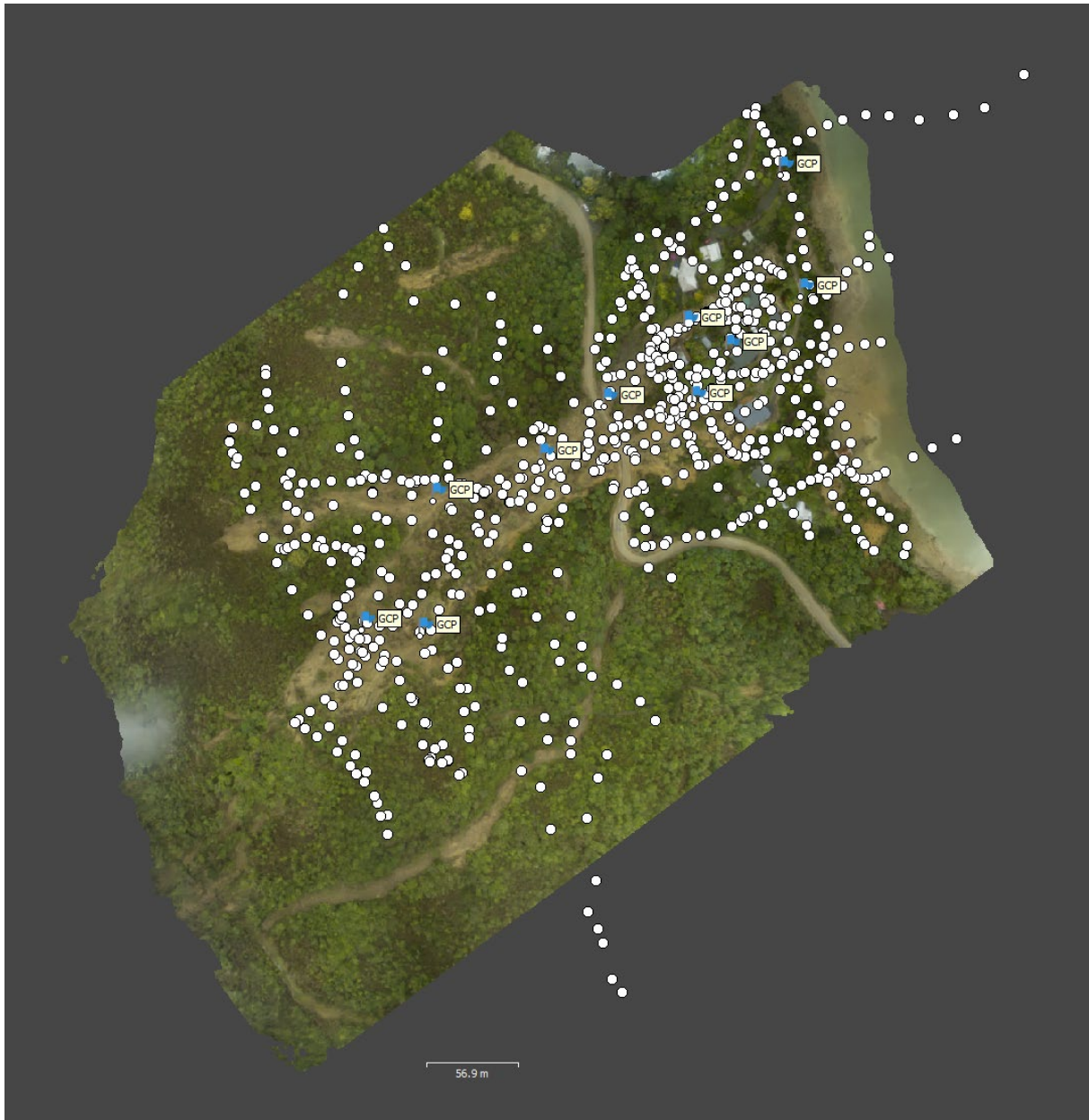
Figure A2.3 LSID3: 723 photos were collected (grey dots); 10 ground control points were used (blue flags).
