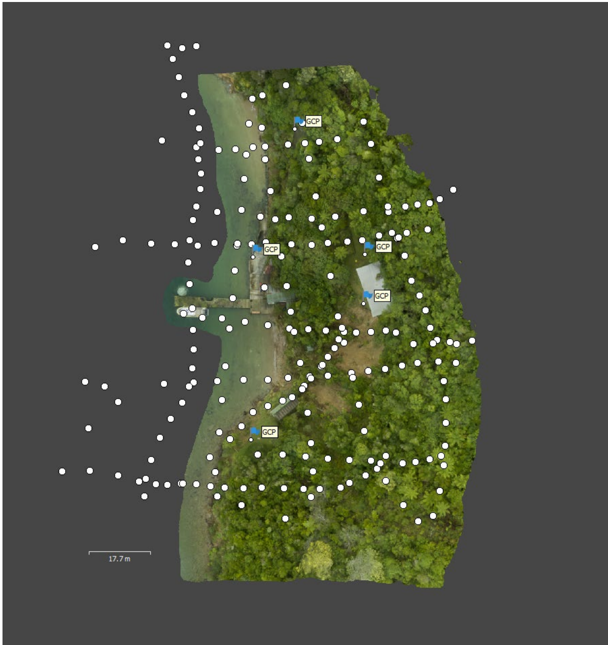
Figure A2.5 LSID6: 216 photos were collected (grey dots); 5 ground control points were used (blue flags).
