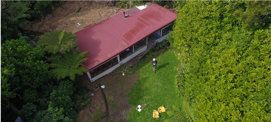
Figure 2.4 Flying the UAV with Aeropoint Ground Control Points (black and white squares), used to georeference the UAV 3D models.
