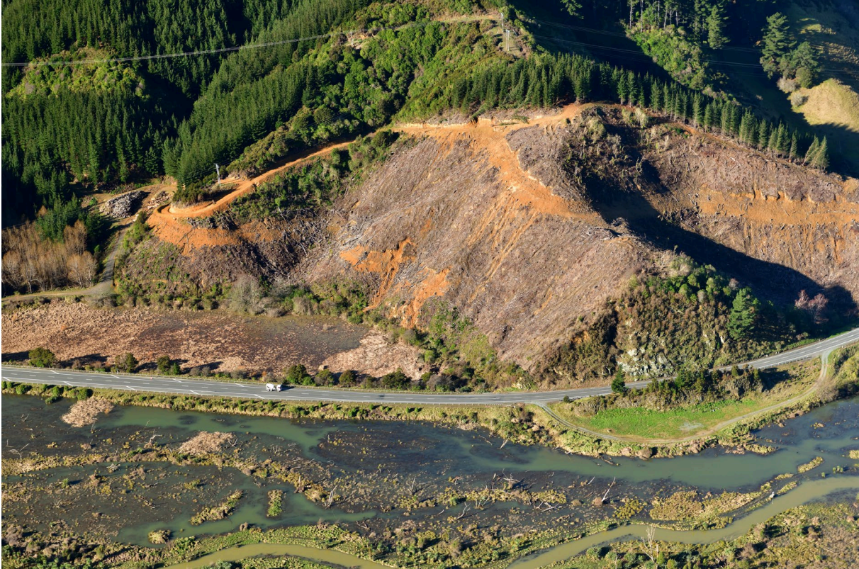
Figure A1.10 Landslides initiated from forestry roads and on newly harvested exotic forest slopes near Para.
