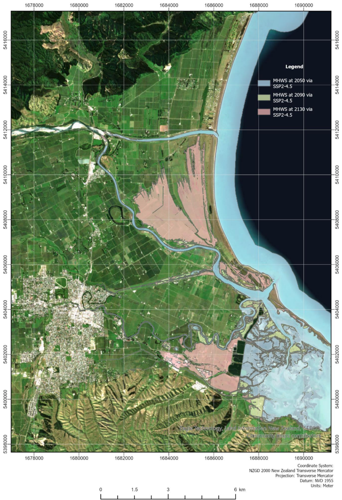
Figure 3-5: MHW direct inundation in 2050, 2090 and 2130 via SSP2-4.5 for the Lower Wairau River Plain.
