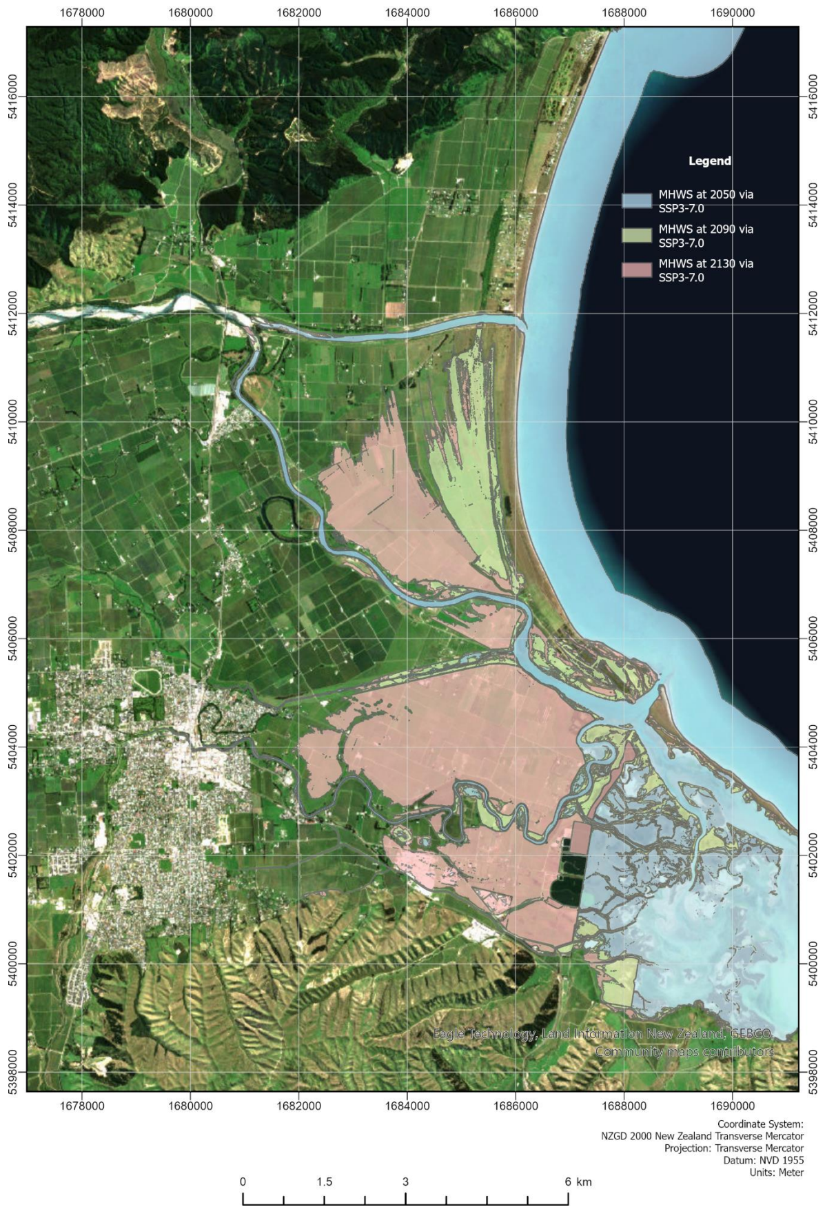
Figure 3-6: MHW direct inundation in 2050, 2090 and 2130 via SSP3-7.0 for the Lower Wairau River Plain.
