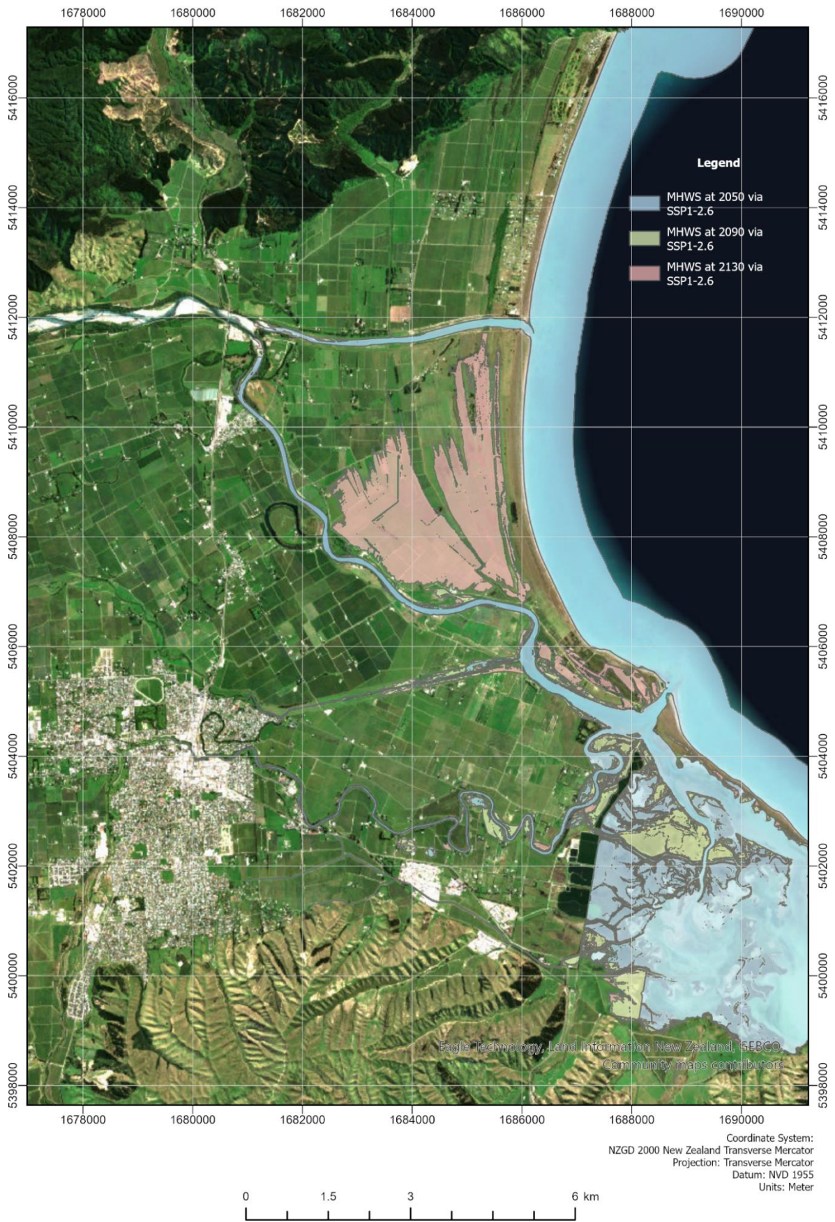
Figure 3-4: MHW direct inundation in 2050, 2090 and 2130 via SSP1-2.6 for the Lower Wairau River Plain.
